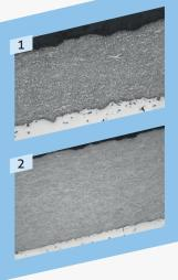
AMS 7882-specified WC-10Co-4Cr in HVOF mode, hardness 1,180 HV0.3, DE 50%, porosity less than 0.5%
